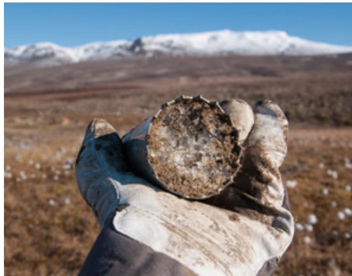
Permafrost drilling: The large drill rig (photo on next page) was used in Zackenberg and at Station Nord in Northeast Greenland in 2012 and 2014. The handheld drill (left side photo) has been used all over Greenland, and it is suitable for drilling within the top 2-4 m. The photo to the right shows a newly drilled core.
